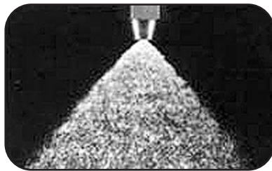
Nozzle spraying additized, high quality heating oil, normally, into combustion chamber
