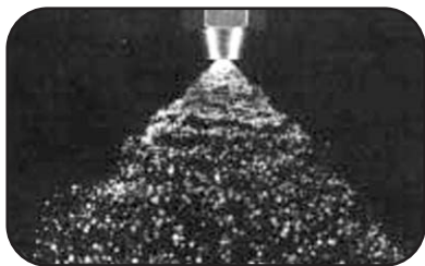
Reduced nozzle spray, caused by deposits from generic, poor quality fuel.
